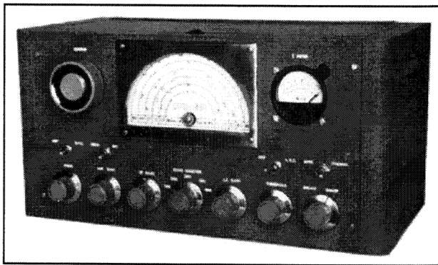
This is W2HBE's 1955 receiver. It included advanced features such as double conversion and mechanical filters. The article is from the October 1955 issue of QST .
